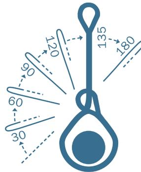
As always, if more than one sling is used and the legs are not vertical, a further reduction in rated capacity must be made for the sling angle.
