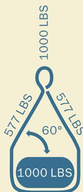
1. Total load is 1,000 lbs. divided by two legs – 500 lbs. load per leg if vertical lift.
