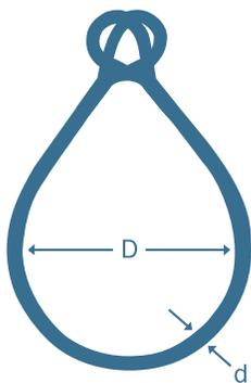
How much the lifting capacity is affected can be calculated by dividing the diameter of the bend where the rope contacts the load (represented by "D") by the diameter of the rope or the component rope diameter in a multi-part sling (represented by "d"). For example, if the diameter of the bend ("D") is 10 and the component rope diameter ("d") is 1/2, the D/d Ratio is  $10 \div 1/2$  or 20.
