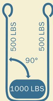
1. Total load is 1,000 lbs. divided by two legs – 500 lbs. load per leg if vertical lift.
